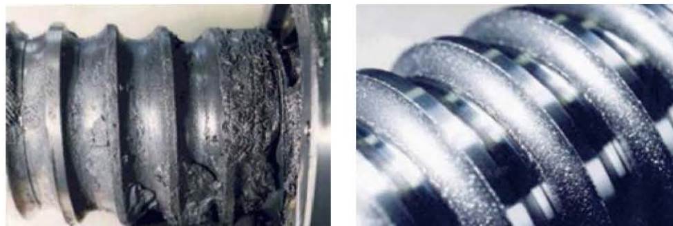
Photo.2 Ball screw damage in the early stage of electric injection molding machines
