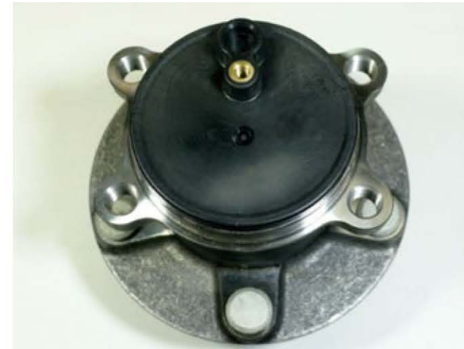
Photo 1 Hub unit bearing sealed by a plastic sensor cap
