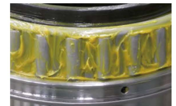
Photo 2 Inside conditions of the bearing with developed grease
